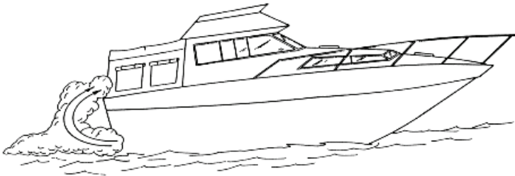
FIGURE 8 INEFFICIENT TRIM ANGLES
